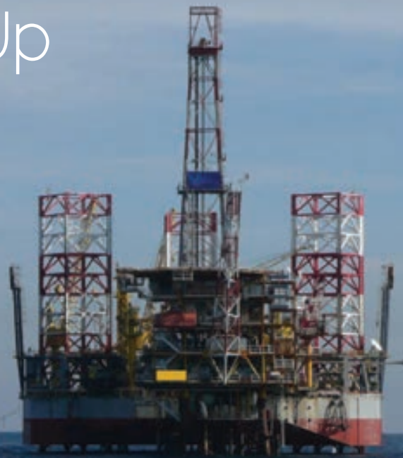
Figure 1. Jack-up drilling rigs are self-elevating structures widely used for oil and gas exploration.
