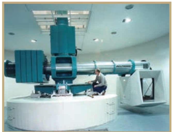
Figure 3. C-CORE's geotechnical centrifuge, capable of producing 200 times Earth's gravity field.
